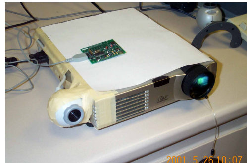
Figure 1. The projector is augmented with a camera and a tilt sensor. (Top) a schematic diagram (bottom) our prototype, with attached camera on the left.
