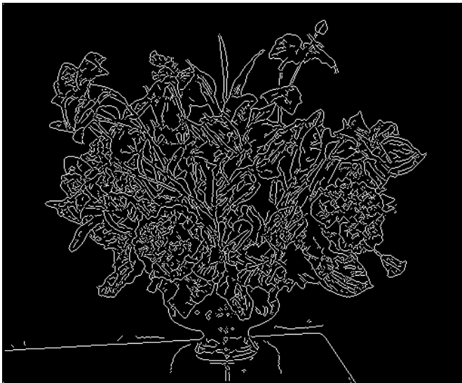
Intensity edges using Canny Edge detector. Notice how a pure intensity image operation leads to spurious edges.
