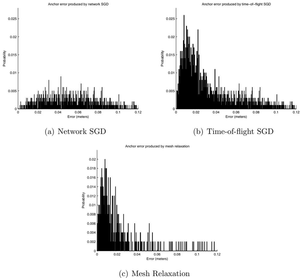
Figure 5-5: Error distributions for anchor nodes localized using spectral graph drawing and/or mesh relaxation in the anchor accuracy tests. All three distributions have heavy tails that have been truncated on the right side of the graph.
