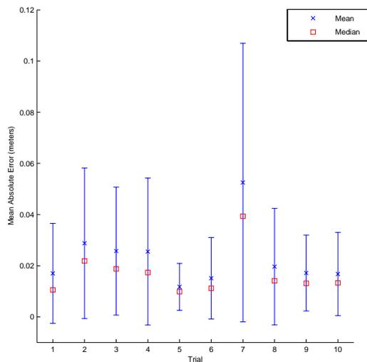
Figure 5-8: Error characteristics for each of ten time-of-flight data sets recorded on the Pushpin hardware test bed using the Pinger v.2. Error bars show one standard deviation from the mean.
