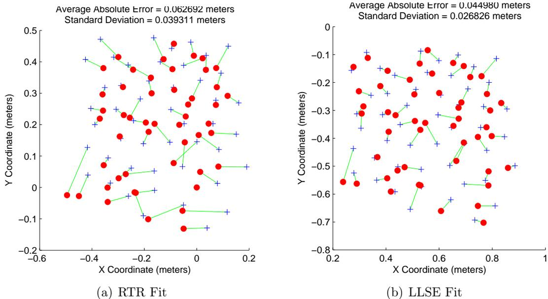
Figure 5-3: Estimated Pushpin coordinates after being fit using a rotation, translation, and possible reflection (RTR fit) or a more general Affine transform that includes scaling and shearing (LLSE fit). The crosses denote measured coordinates and the circles denote coordinates estimated using lateration. The line connecting each cross to a circle indicates which estimated coordinate corresponds to which measured coordinate.
