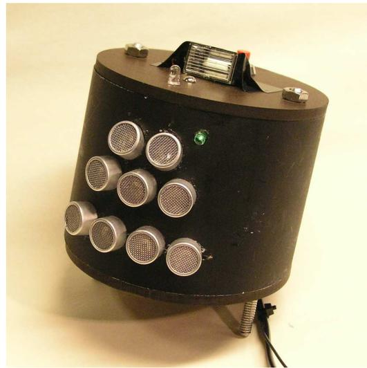
Figure 2-7: The “Pinger” device simultaneously generates a flash of light and a 40-KHz ultrasound pulse at the push of a button. By measuring the time difference of arrival between these two signals and dividing by the speed of sound in air, a Pushpin node can measure its distance to the Pinger to within about 1-cm.
