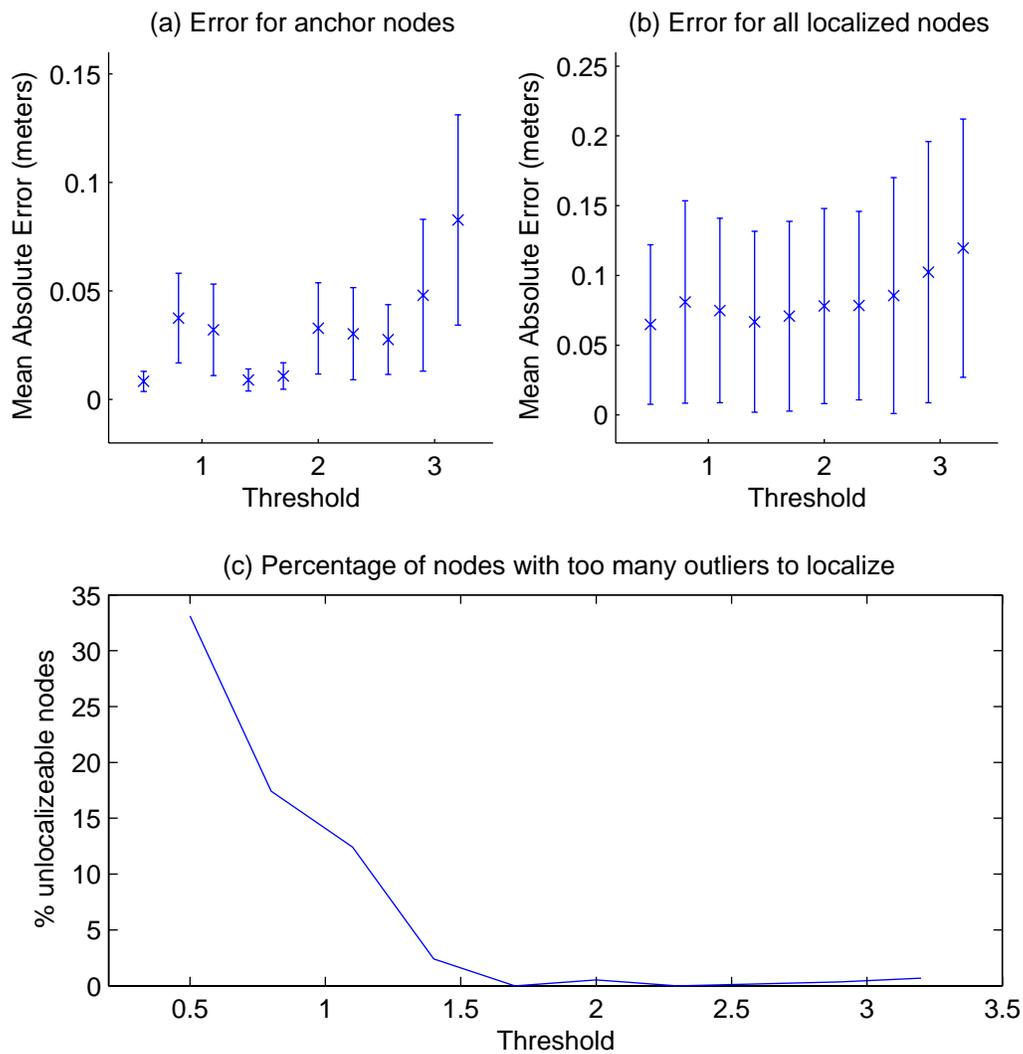
Figure 5-9: The effects of a preprocessing step that rejects outlying time-of-flight measurements. The threshold for rejection is the number of standard deviations from the norm of a node's neighbors' measurements.
