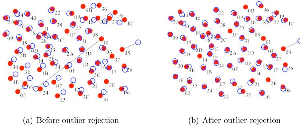
Figure 5-10: Coordinate outlier rejection is critical for selecting and rejecting nodes whose coordinates grossly disagree with their neighbors', such as node 01 in figure (a) above. Figure (b) shows the network after 01 has been automatically rejected. However a minor outlier, namely node 05, was missed on this pass.
