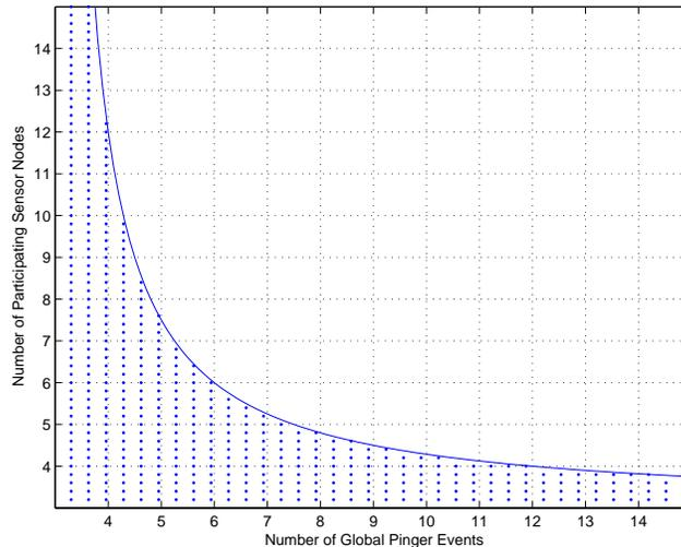
Figure 3-1: There is an inherent trade-off between the number of nodes participating in localization and the number of global Pinger events required to find a localization solution. The line represents a lower bound on the number of Pushpins and Pinger events required for a solution to exist. The actual number needed for a rigid solution falls somewhere outside of the shaded region.
